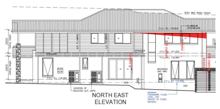
The non-compliance is partially due to the requirement for the dwelling to achieve a minimum floor level due to an overland flow issue.
