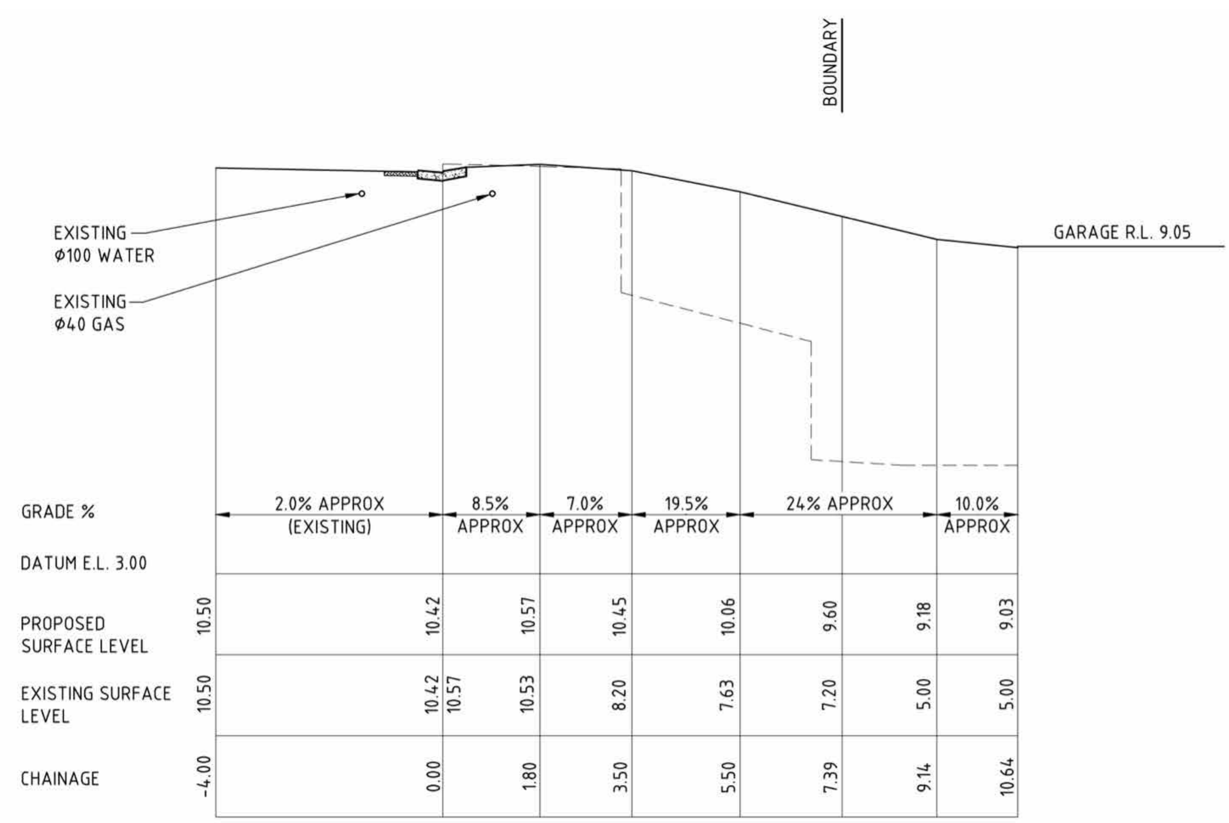
NEW DRIVEWAY LONGSECTION - GARAGE FFL: 9.05
