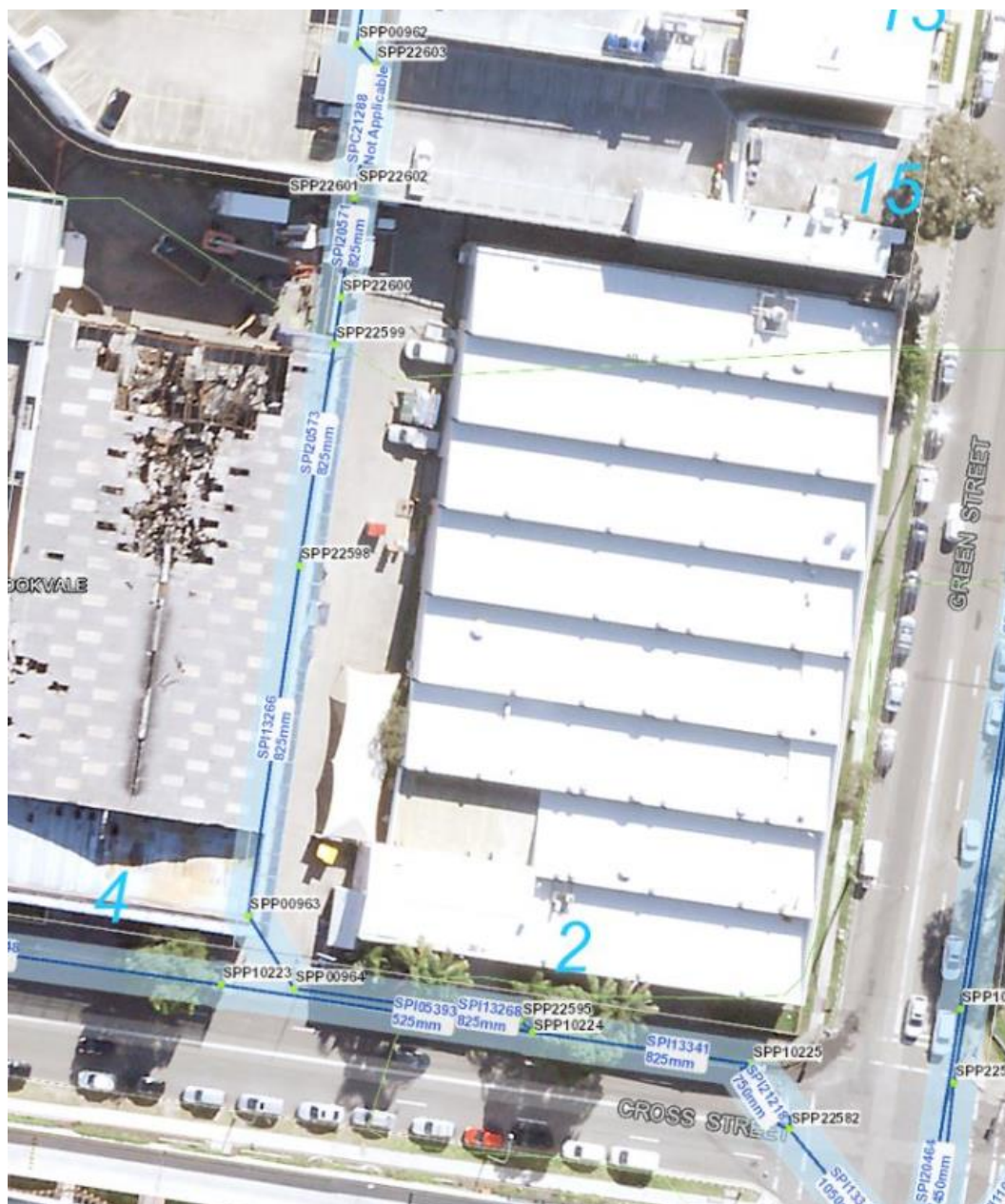
Figure 2-2 Stormwater Pipe Network (Northern Beaches Council)
