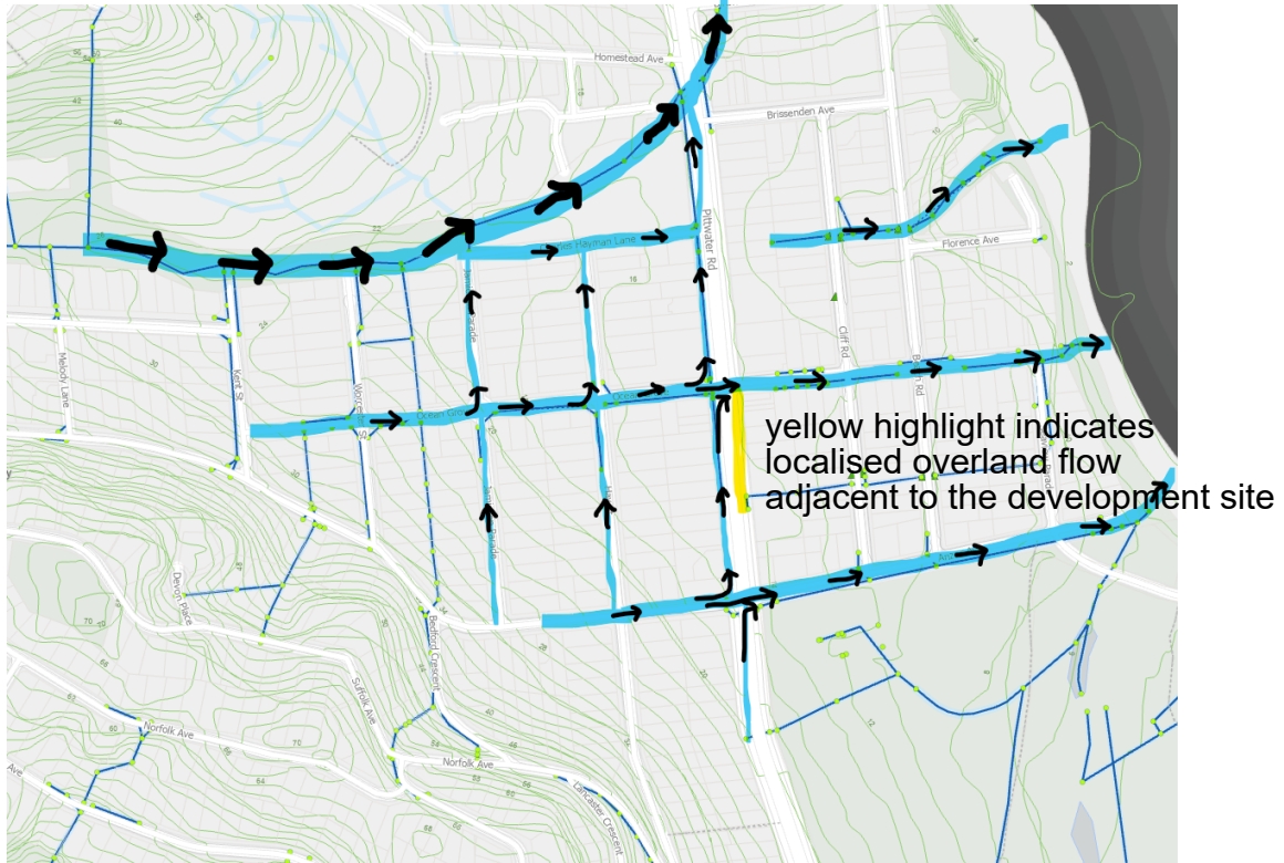
Surrounding / uphill catchment + associated indicative overland flow paths (Northern Beaches Council web site / Barrenjoey Consulting Engineers pty ltd)
