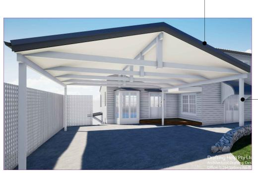
**NEW TIMBER FRAMES** DOUBLE CARPORT WITH COLOURBOND ROOF. TO BE BCA AND NCC COMPLIENT
