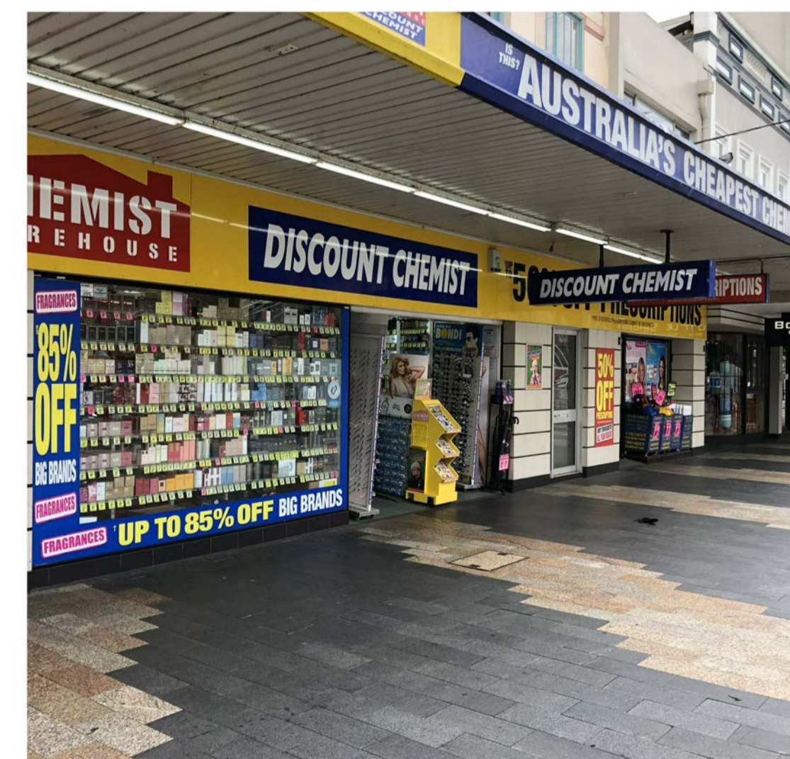
Allow to repaint entire façade and masonry returns to The Corso in heritage colour scheme based on paint scrape evidence performed on site once access to façade is provided. Paint shall be Dulux Acratex Acraseal or similar to heritage architect's approval.
