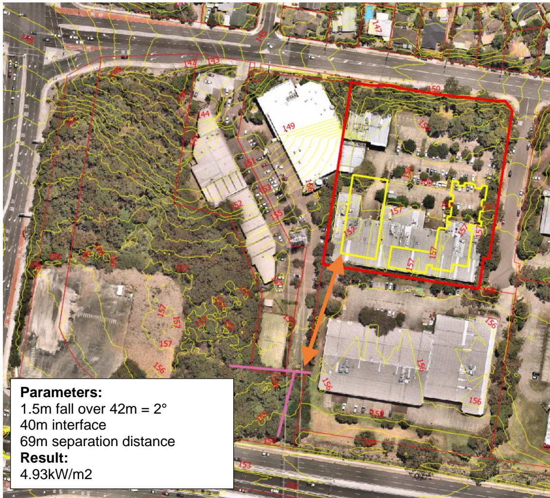
Figure 10: Aerial view of the subject area, 1 metre contours and Transect 4 Subject site (thick red outline) and proposed building envelope (yellow outline)
