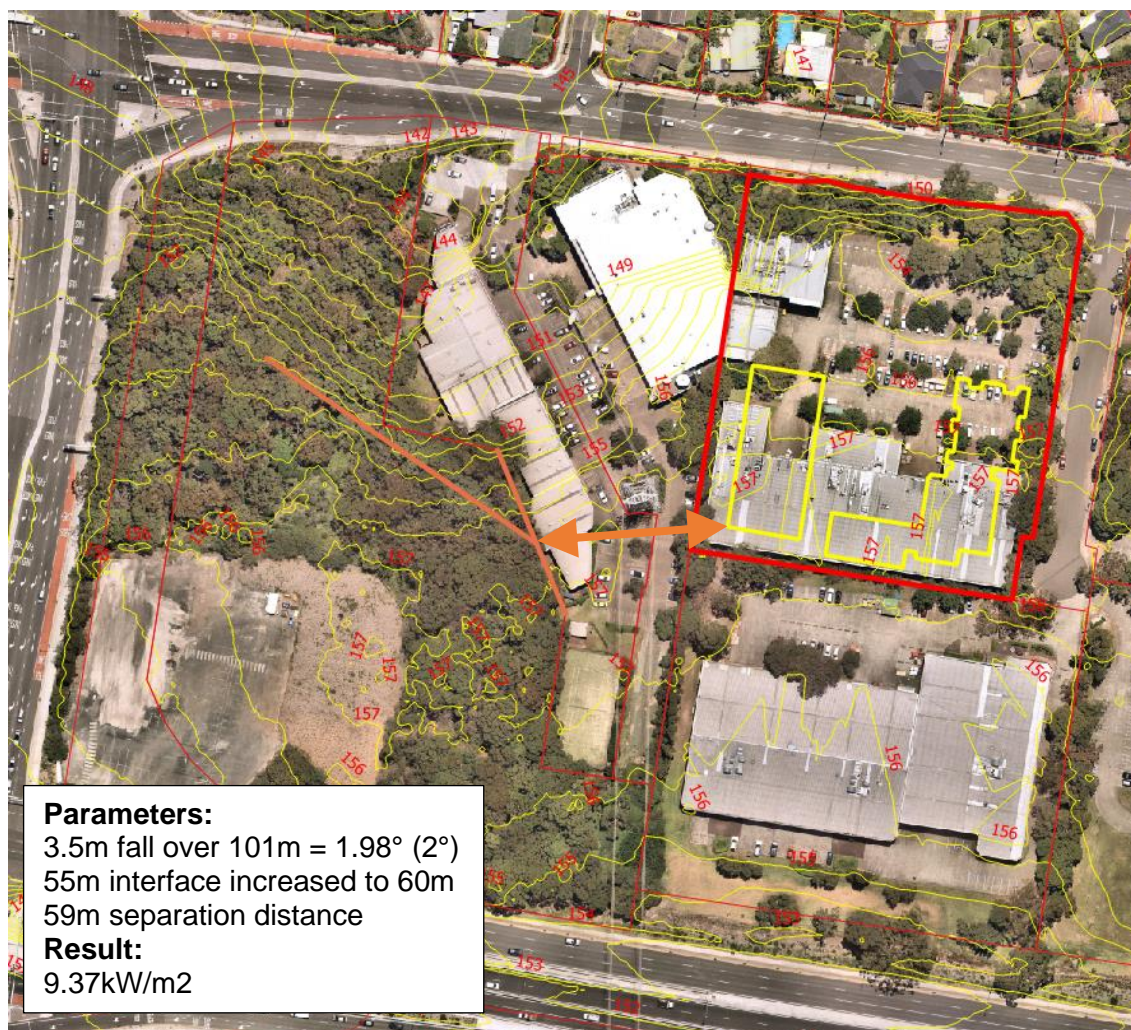
Figure 07: Aerial view of the subject area, 1 metre contours and Transect 1 Subject site (thick red outline) and proposed building envelope (yellow outline)
