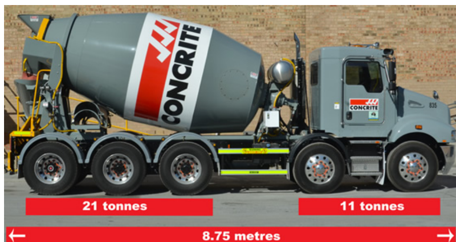
Photograph of a typical concrete delivery truck that will be utilised during the concrete pour phase
