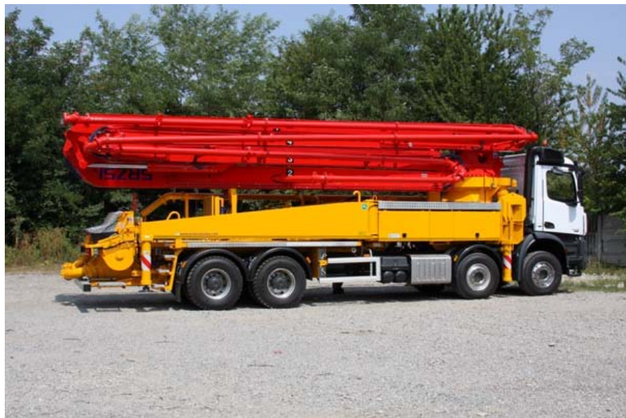
Photograph of a typical 51m concrete boom pump that will Be utilised during the concrete pour phase
