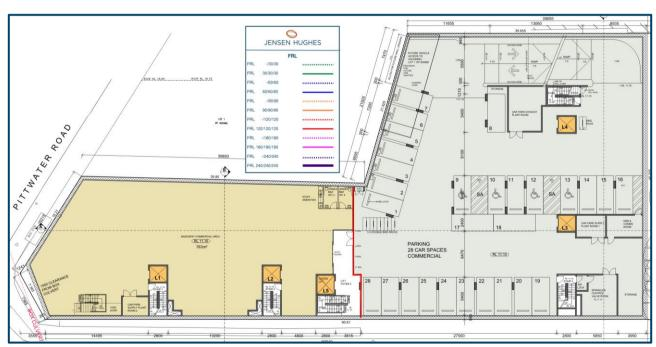
The main switchboard location shown in Basement Level B1. If the switchboard is required service emergency equipment required to operate in an emergency, the switch room is to have an FRL of 120/120. The design of the switch room is such that compliance can be readily achieved.
