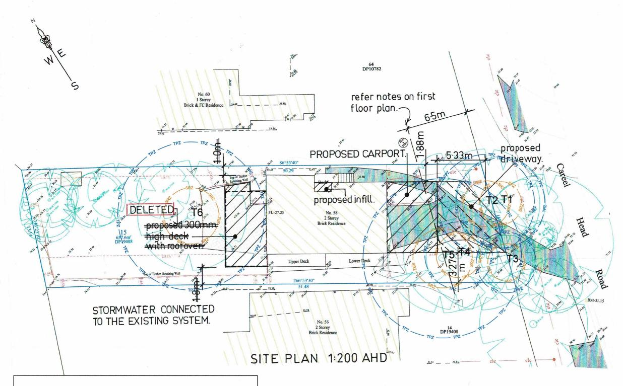
TPZ & SRZ PLAN WITH TREE PROTECTION ZONES AND STRUCTURAL ROOT ZONES SHOWN TO SCALE.
