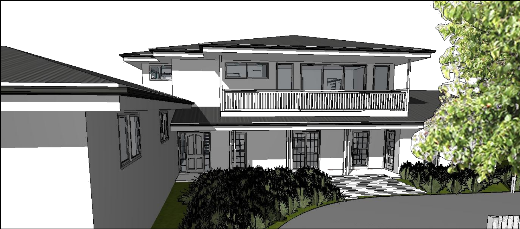
MT-01 PAINTED COLOURBOND METAL ROOF SHEETING. 'IRONSTONE' OR SIMILAR TO MATCH EXISTING. WHERE MARKED ON ELEVATION.
