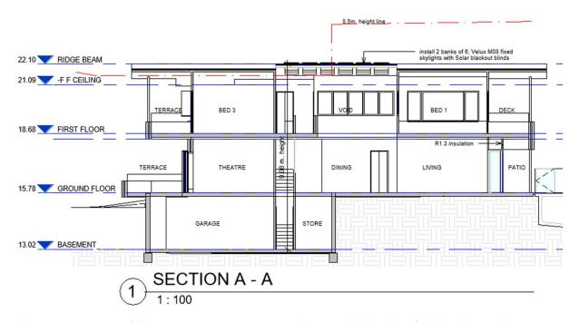
This is section A-A of the DA drawings Revision A, showing the height of the building relative to the previously excavated, 2004, basement level.
