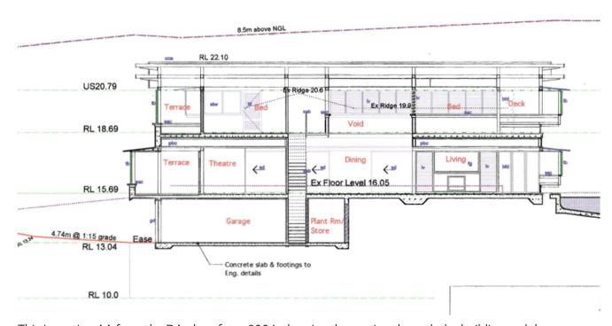
This is section AA from the DA plans from 2004, showing the section through the building and the building height line relative to the existing ground line at that time.
