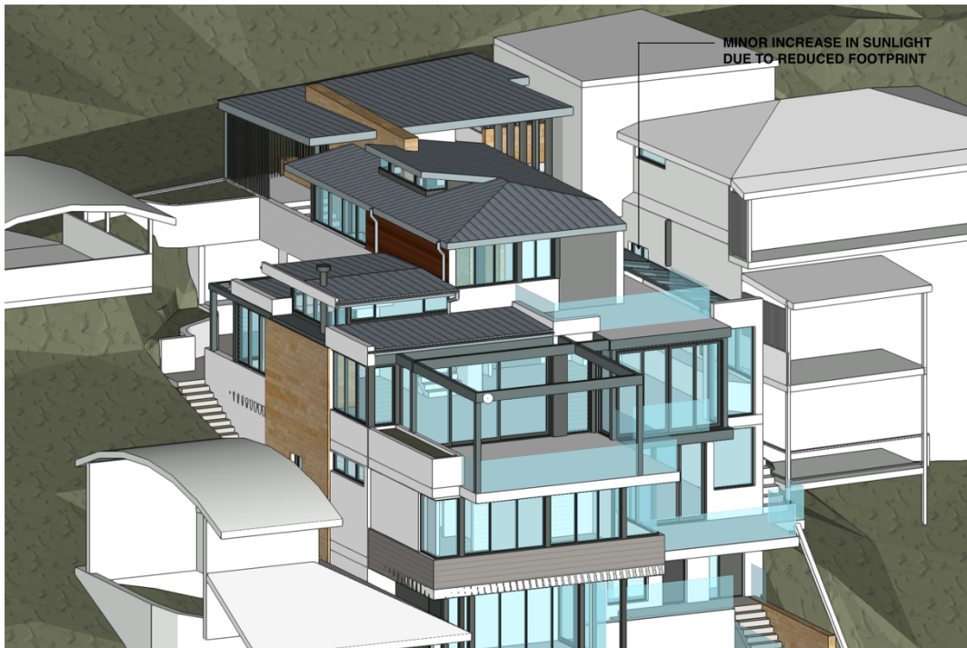
Diagram 1: Diagram showing what is illuminated by the sun at 3:30 PM on June 21. Design with reduced first floor footprint results in only a tiny increase in sun.
