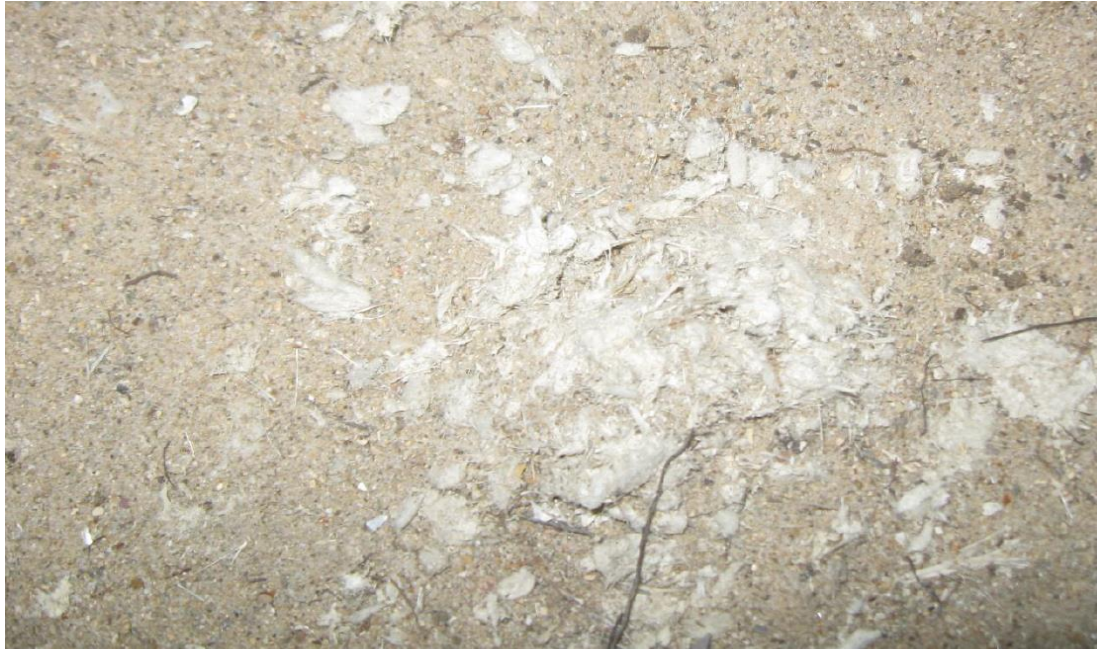
Photograph 7: B00G, exterior, subfloor, throughout, loose fibre in sand/soil, asbestos detected by analysis
