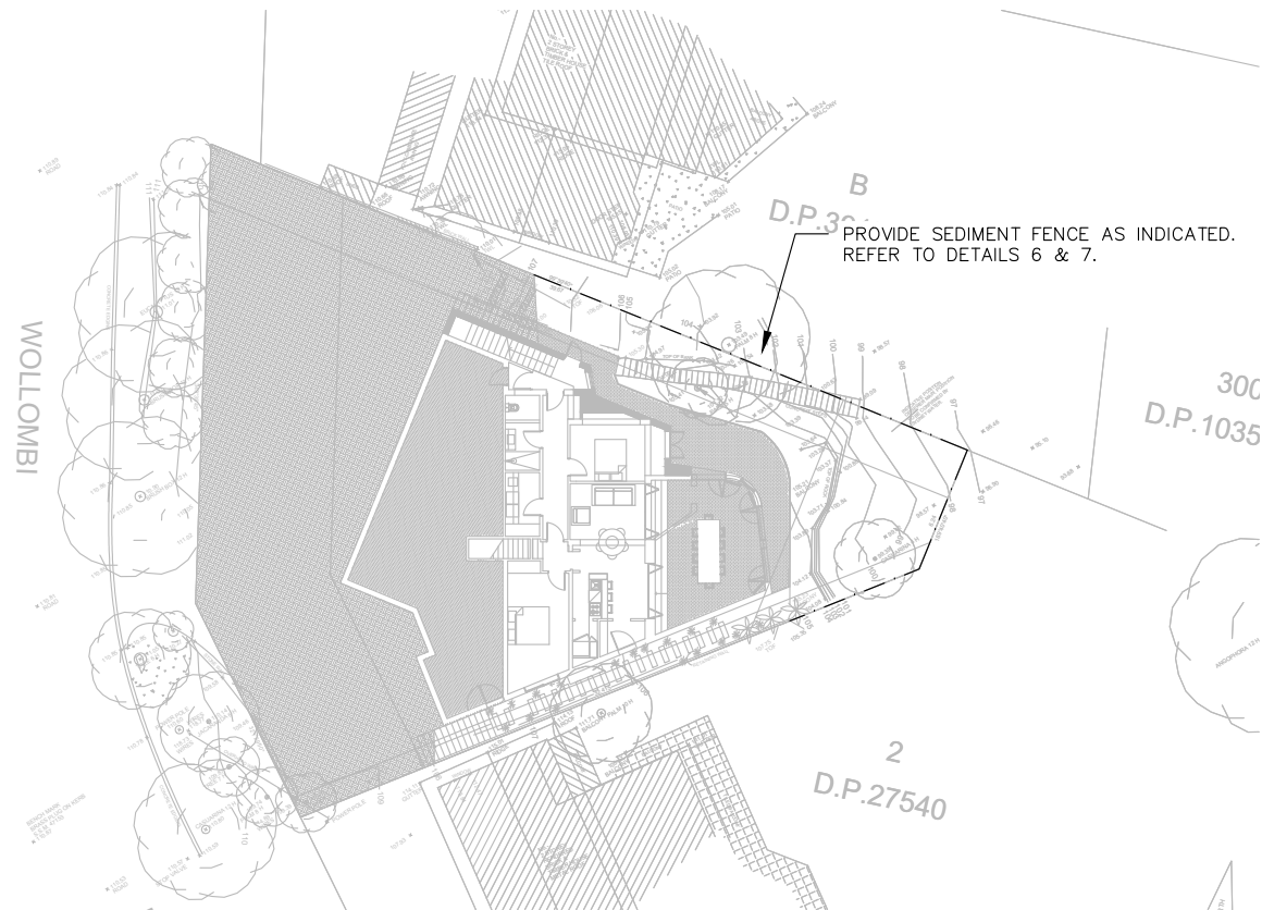
PLAN 8 SEDIMENT & EROSION CONTROL PLAN—LOWER GROUND FLOOR LEVEL 1: 400
