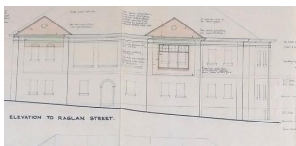
Figure 13 1971 working drawing indicating the 'bricking in' of the Raglan St observation deck and installation of windows (Unknown Author provided by Northern Beaches Council)
