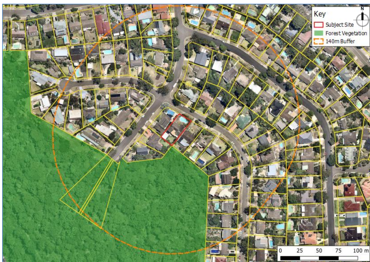
Figure 5. Hazardous vegetation affecting the subject building. Source: NearMap (2019) with overlays by BFCS P/L
