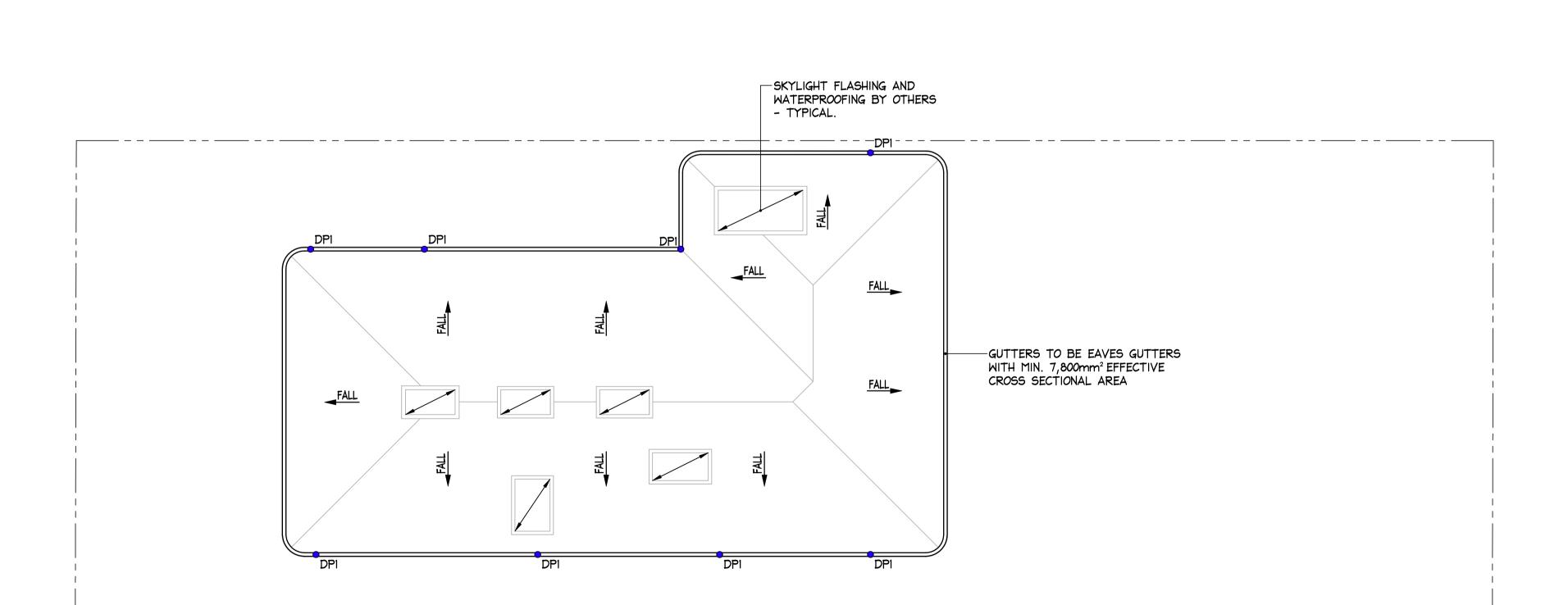
FIRST FLOOR STORMWATER DRAINAGE PLAN
