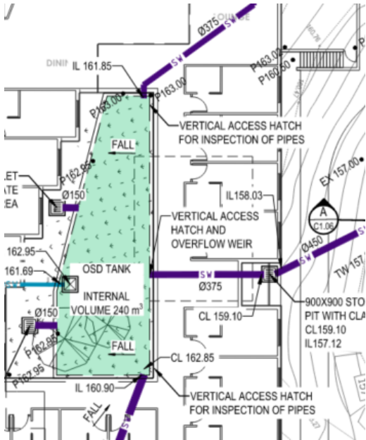
ACOR OSD Location beneath building
