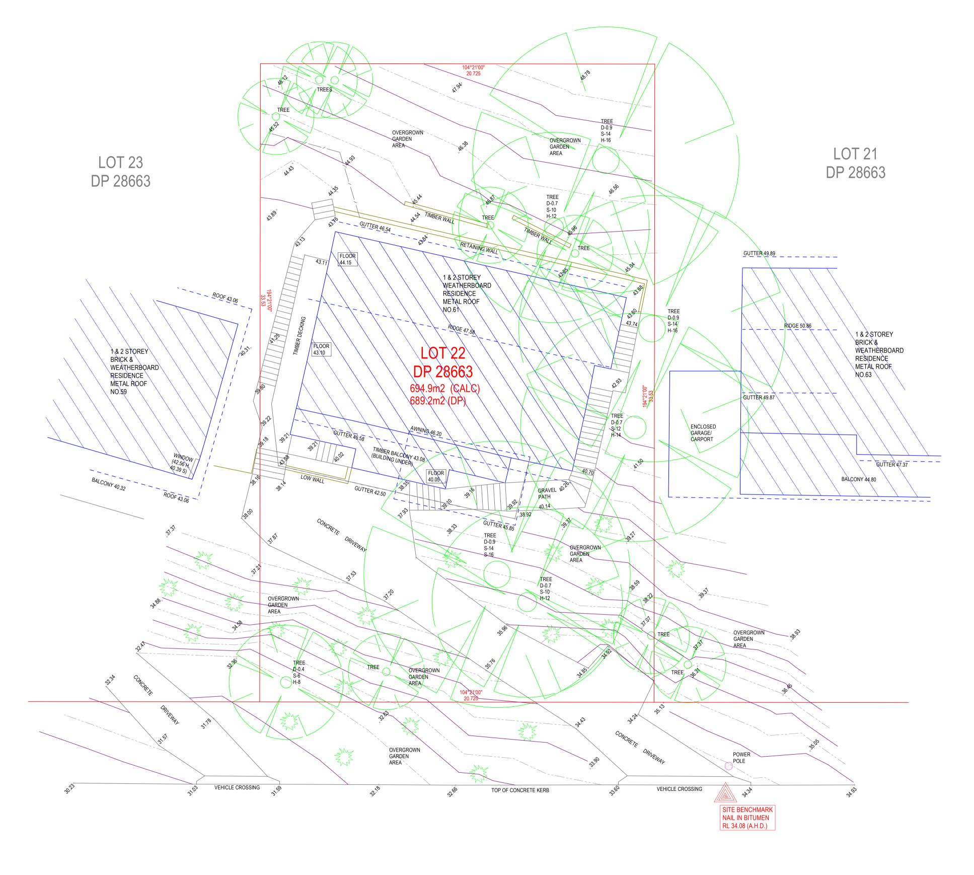
1. LEVELS SHOWN ARE TO AUSTRALIAN HEIGHT DATUM. ORIGIN OF RL'S; SSM 40963 - RL 48.78 (A.H.D.) 2. BEARINGS ARE ON MM NORTH AS DERIVED BY DP 28663. BOUNDARIES OF THE SITE HAVE BÈEN DÉFINED BY SURVEY. 3. RELATIONSHIP OF IMPROVEMENTS AND DETAIL TO BOUNDARIES IS DIAGRAMMATIC ONLY AND SPECIFIC DETAILS, IF CRITICAL, WILL REQUIRED A FURTHER SURVEY - UNLESS OTHERWISE SHOWN.
