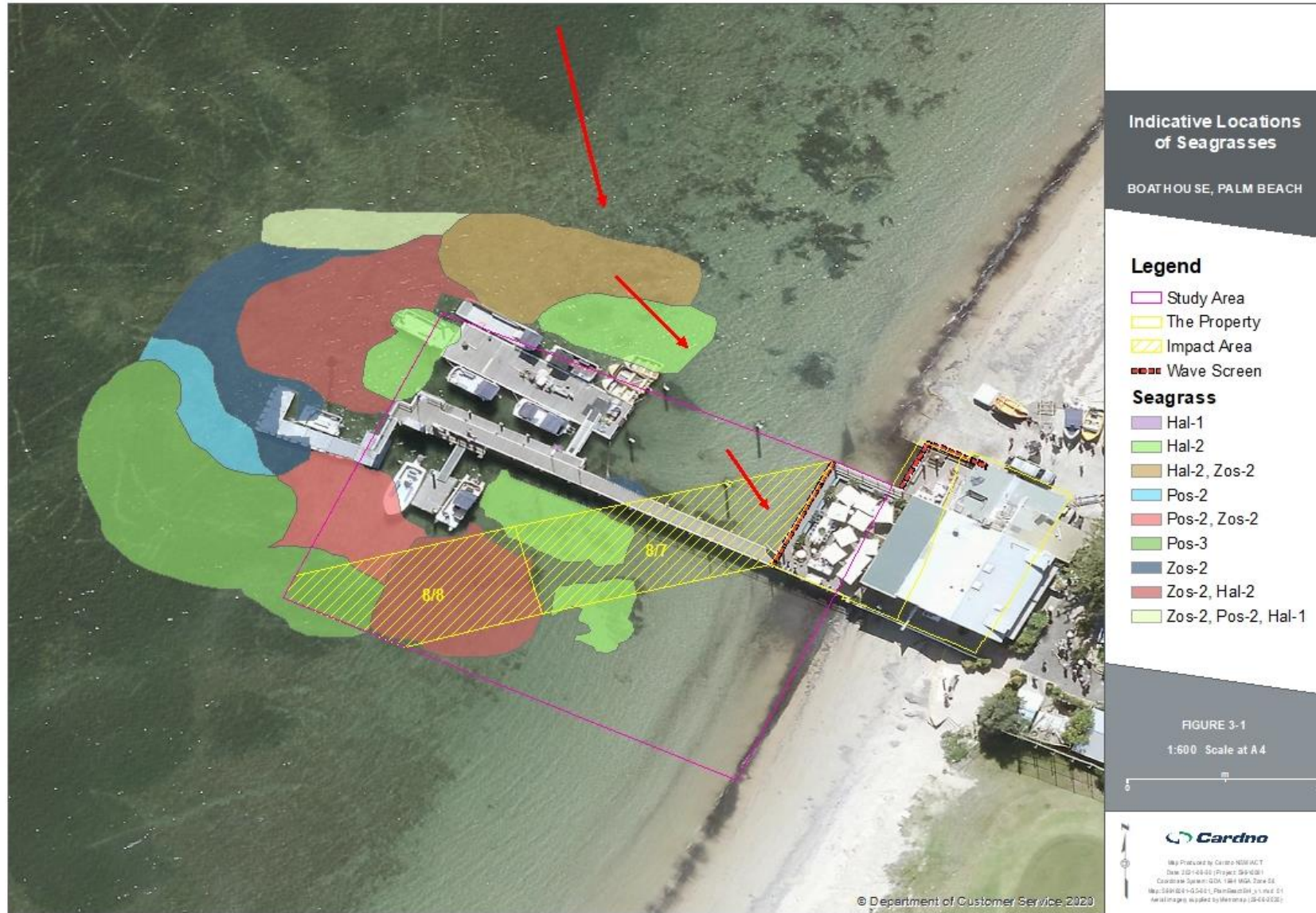
Figure 3-1 Aerial figure of the Property with the indicative location of seagrasses present within the Study Area at the time of the survey. Wave screen impact 8/8 and 8/7 zones highlighted in yellow. The red arrows indicate the recommended path for the barge movements to avoid areas of Posidonia .
