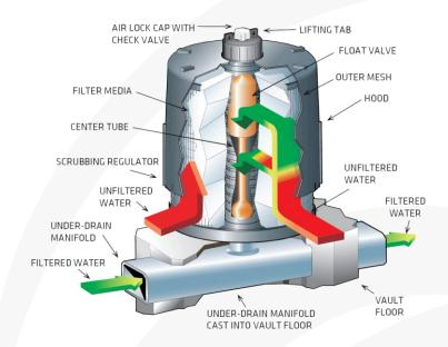
As the rain event subsides, the water level outside the cartridge drops and approaches the bottom of the hood, air rushes through the scrubbing regulators releasing the water column and breaking the siphon. The turbulent bubbling action agitates the surface of the cartridge promoting trapped sediment to drop to the chamber floor. After a rain event, the chamber is able to drain dry by way of an imperfect seal at the base of the float valve.
