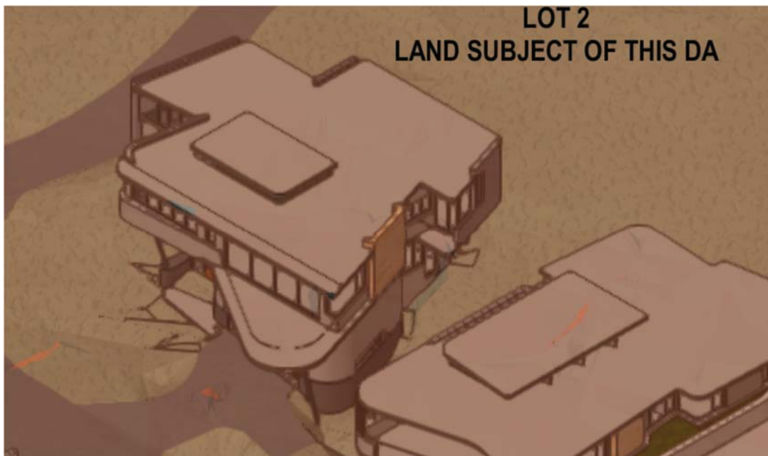
Figure 22 – 3D 8.5m building height plane over site (fully complies)
