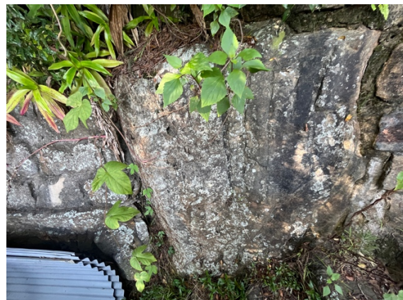
Photo 6: Outcropping bedrock with detached block joints in the general area of the proposed driveway works
