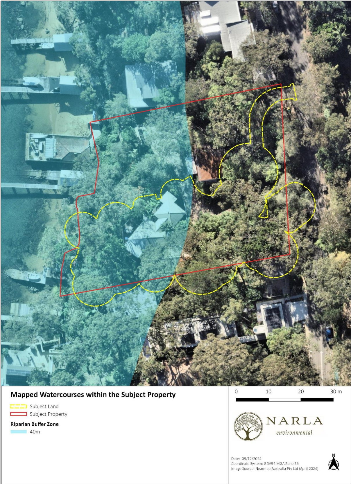
Figure 7. Watercourses and riparian buffer zones occurring within and adjacent to the Subject Land.
