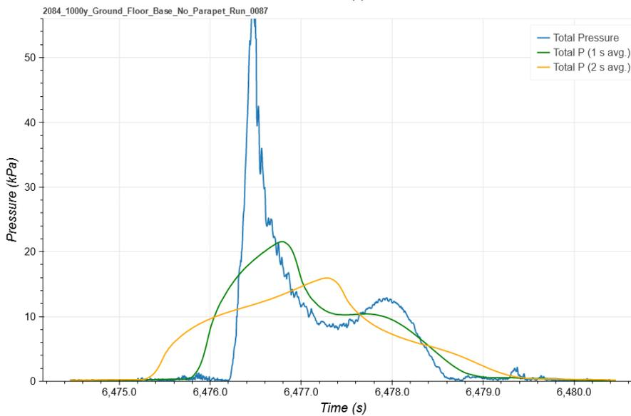
Figure 6.7 New building without parapet, 1000 year ARI, 2084, lower floor bottom
