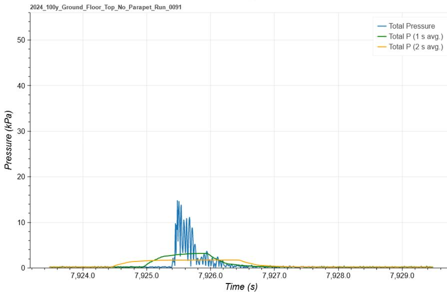
Figure 6.2 New building without parapet, 100 year ARI, 2024, lower floor top
