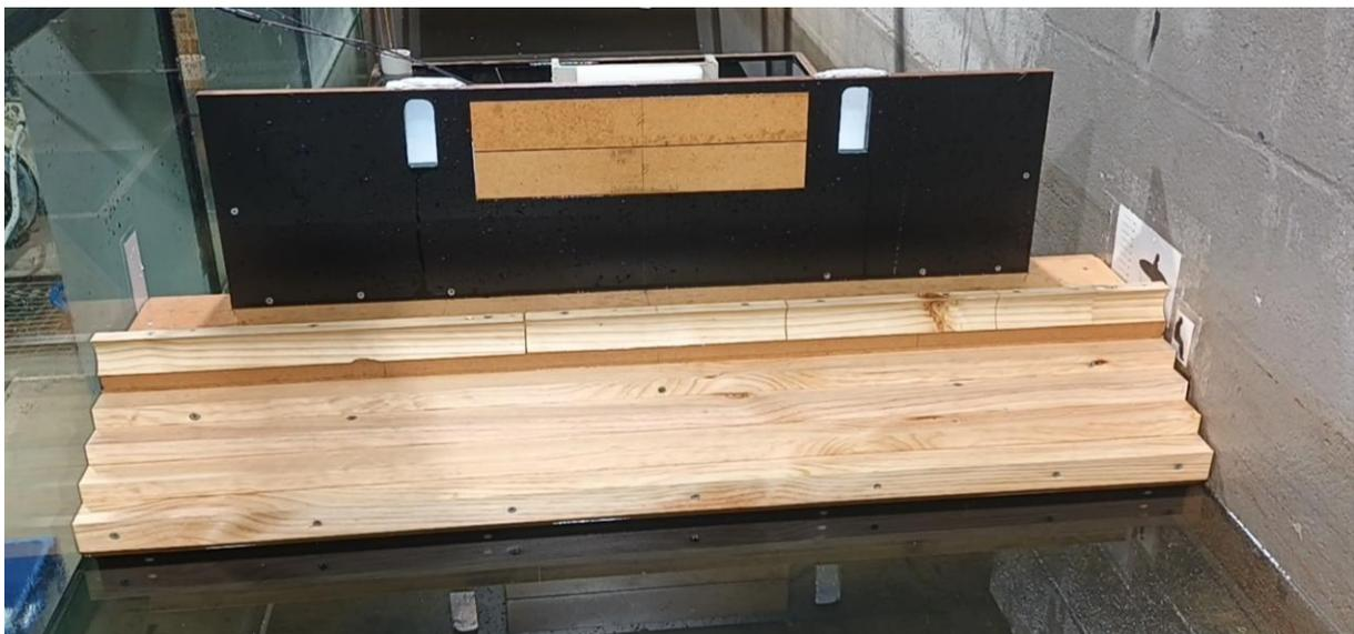
Figure 2.2 Upper floor top and upper floor bottom load cell panels and two window openings
