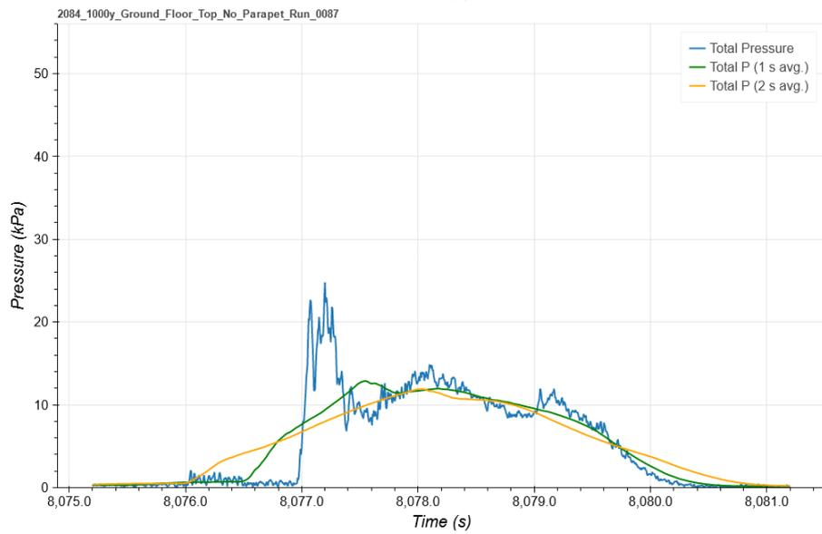
Figure 6.8 New building without parapet, 1000 year ARI, 2084, lower floor top
