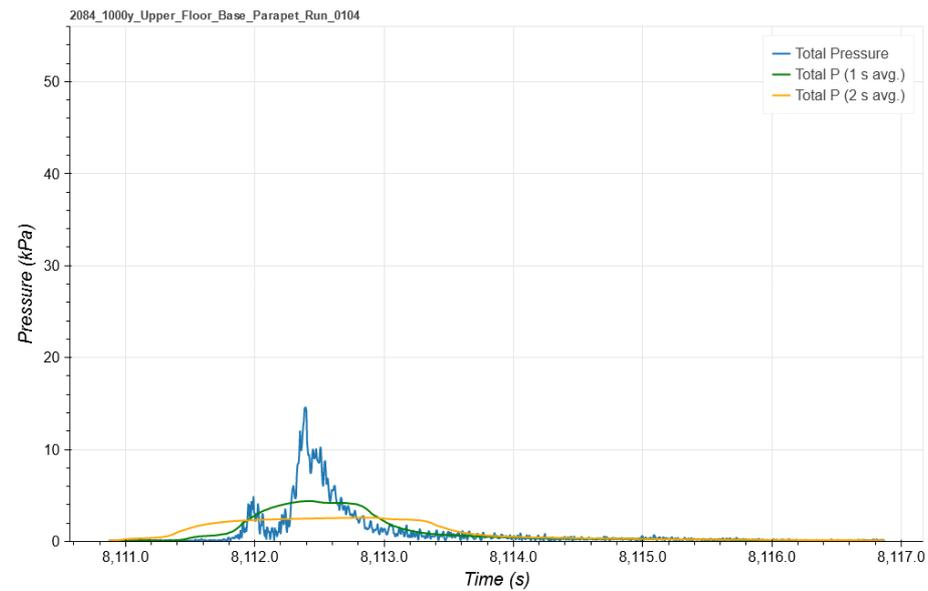
Figure 5.15 Existing building with parapet, 1000 year ARI, 2084, upper floor bottom
