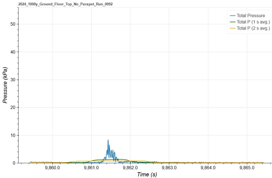
Figure 6.5 New building without parapet, 1000 year ARI, 2024, lower floor bottom
