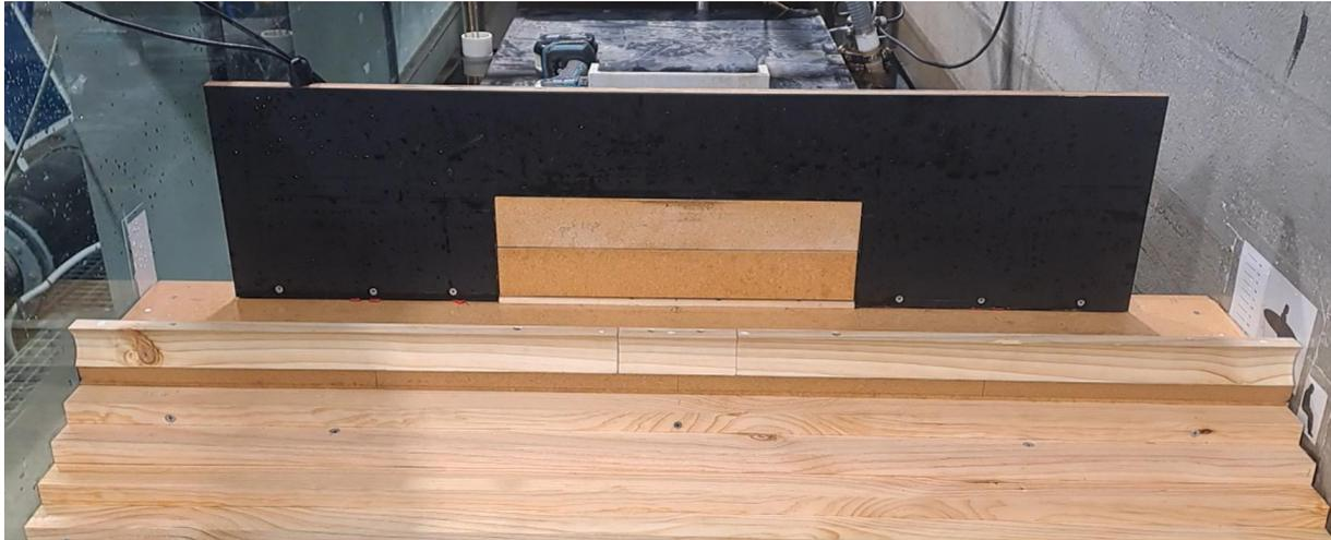
Figure 2.1 Ground floor top and ground floor bottom load cell panels
