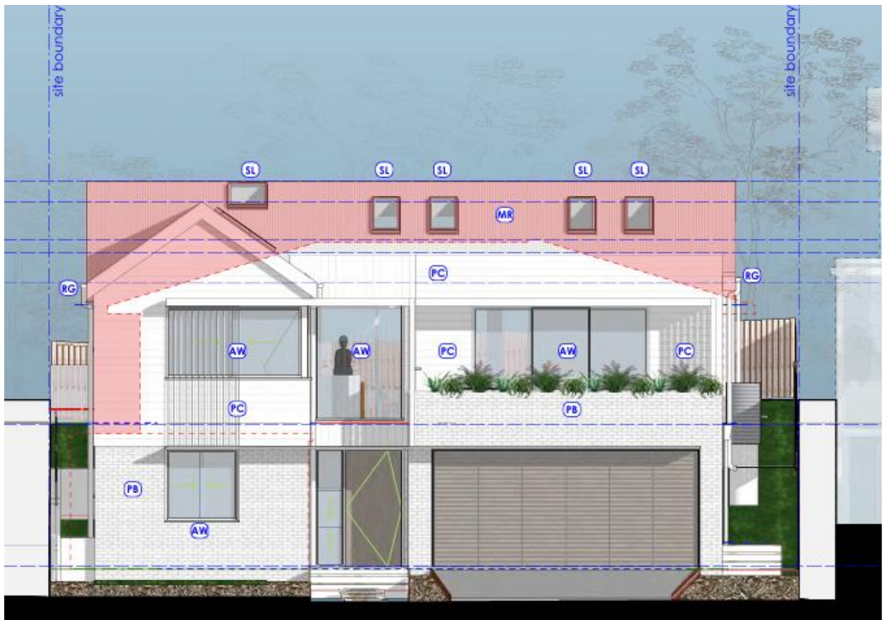
Figure 12. Extract – Front Elevation - wall height of 5.530 m
