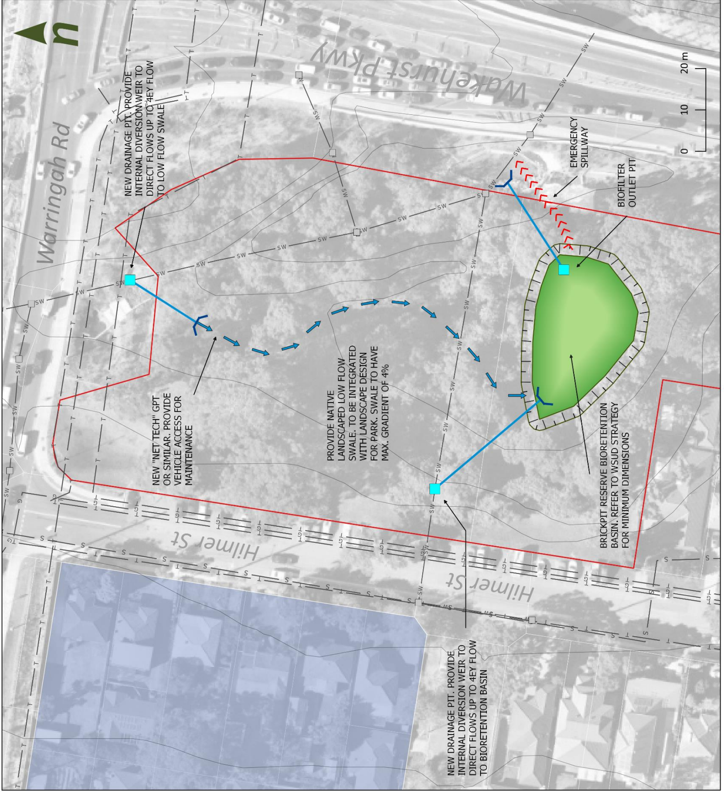
Figure 8-2 - Brickpit Reserve WSUD concept
