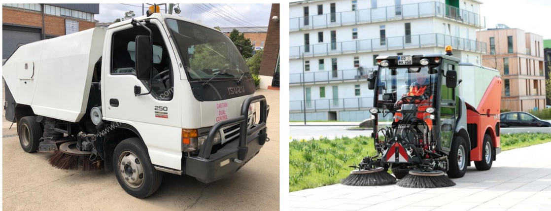
Figure 7-1 Mechanical street sweeper (LHS) and footpath sweeper (RHS)
