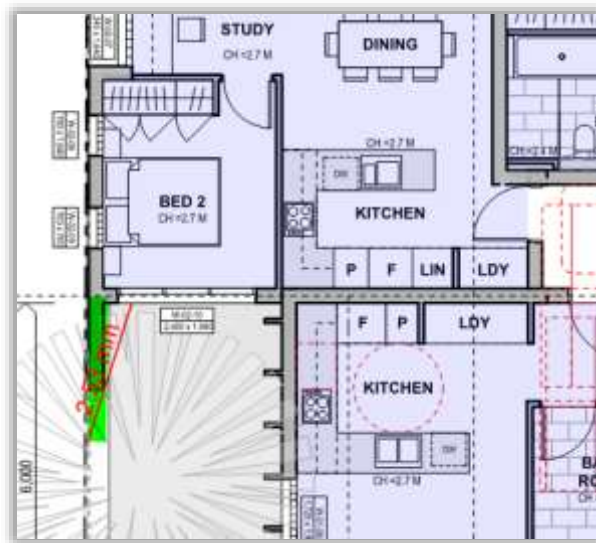
Figure 4 – Blade wall modifications to ensure the bedroom window in units 2,16 & 30 are greater than 3m from the side boundary fire source feature
