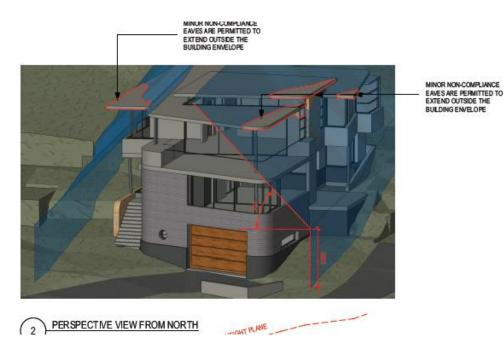
Figure 26 – building envelope compliance (NW boundary)
