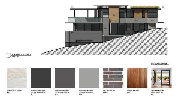
Figure 15- proposed north-west elevation of House 4 and schedule of colours and materials
