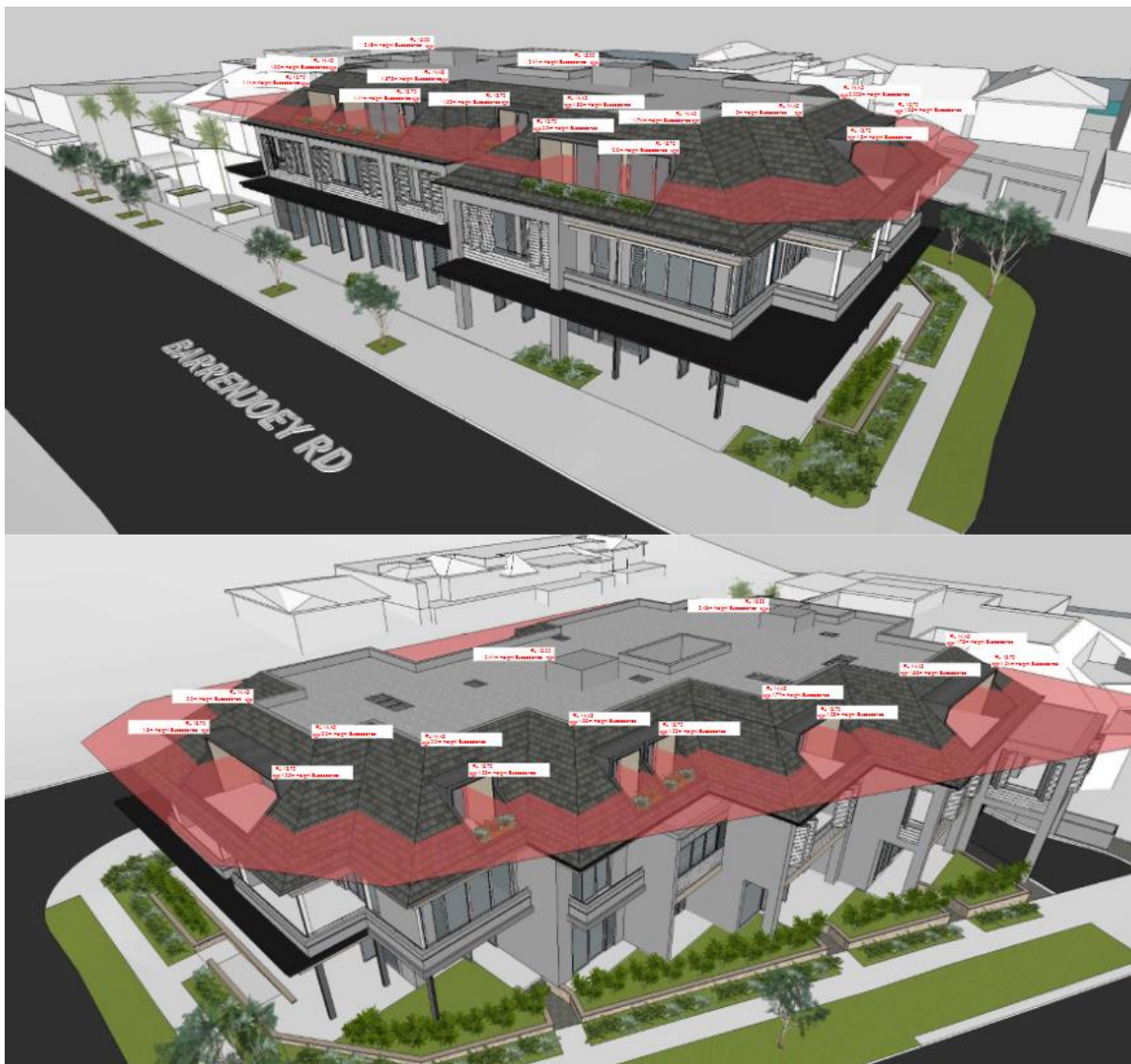
Figure 1 - Plan extract showing height breaching elements above the 8.5 metre height standard depicted by pink blanket layer
