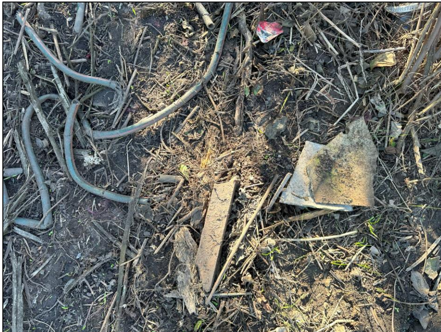
Photograph 6.10.1 Localised suspected asbestos fibre cement surficial impacts within the southern portion of the site, as observed on 21 June 2023.
