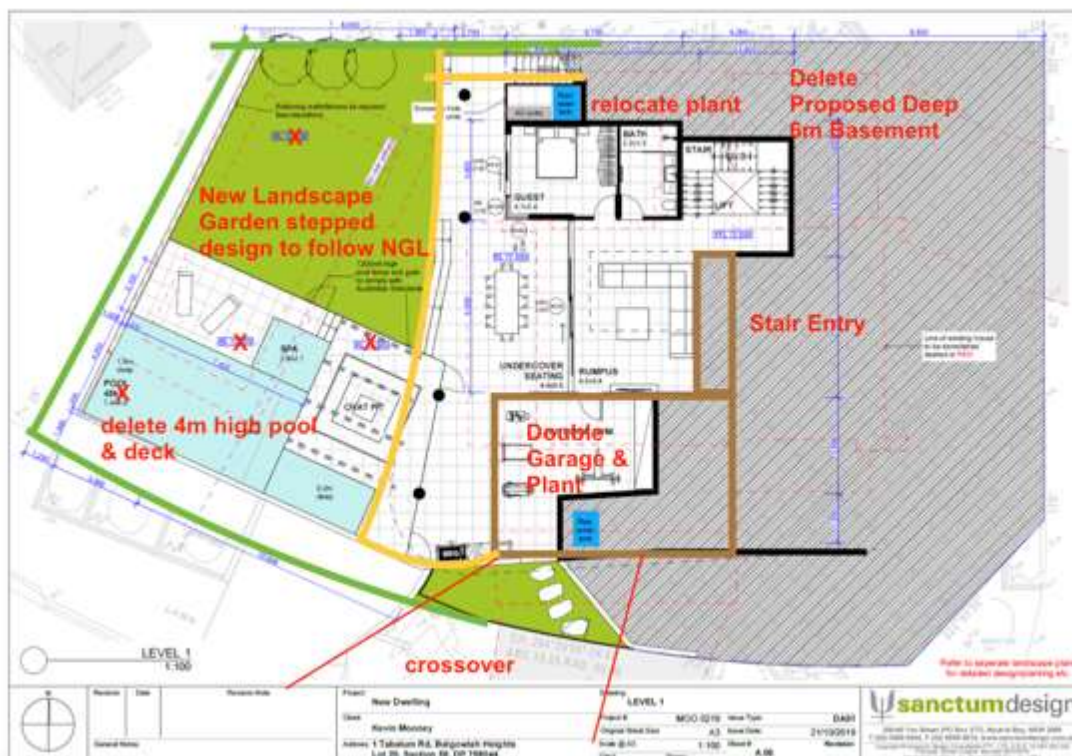
Alternative New Landscape Garden to follow Ground Levels [Existing] . Pool to MDCP controls set within landscape at ngl grades from Level 1 to RL 68.87. Garaging at Level 1 is similar location to existing. New stair entry passageway from garage. Delete entire 6m deep basement and 4m high pool and 4m+ high decks adjacent 6 Cutler. New crossover.
