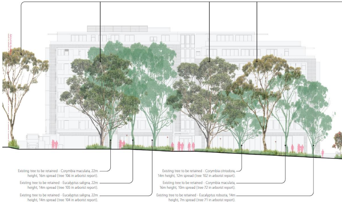
Figure 7: Cross section of Skyline Place elevation showing screening provided by canopy trees (Source: Paddock Studio)
