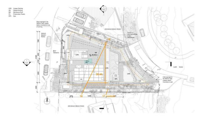
Marked-up Roof Plan: Zone in excess of 8.5m building height: the excessive height above 8.5m is not 'minor' and fails LEP 4.3 2D [a], and fails the objectives LEP 4.3 [1] [a] desired character of locality, [b] compatible with neighbours, [c] overshadowing, and [d] view.
