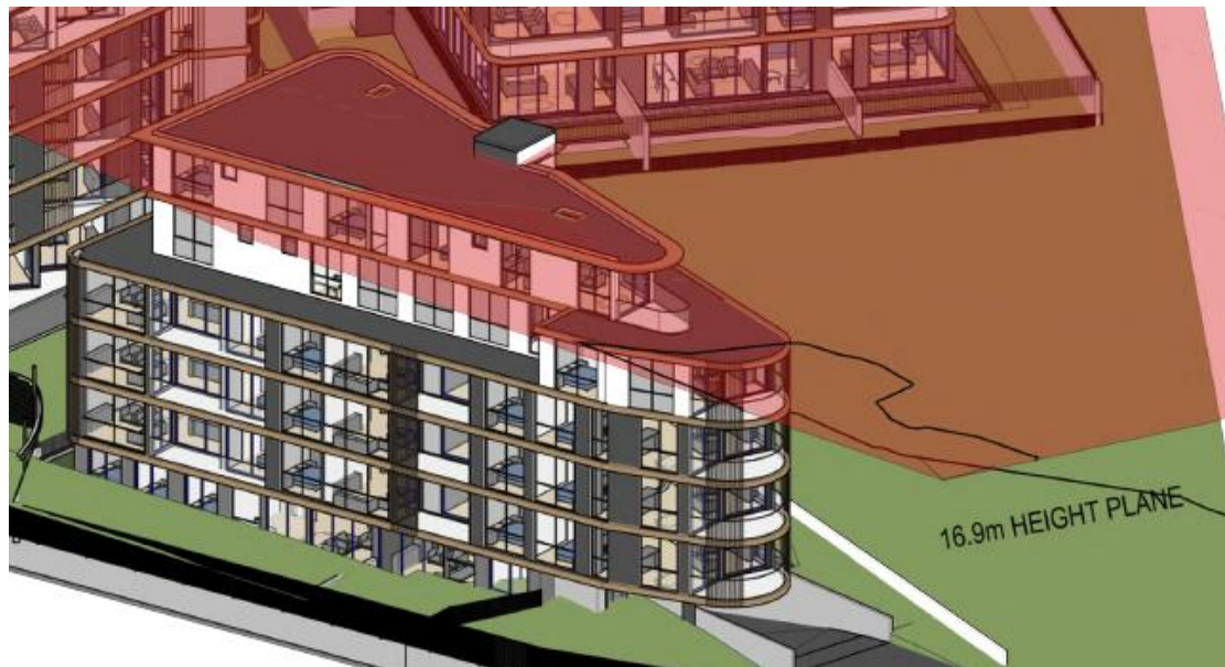
Figure 2 – Plan extract of 16.9 metre building height blanket diagram depicting minor non-compliant projecting elements on Building C.
