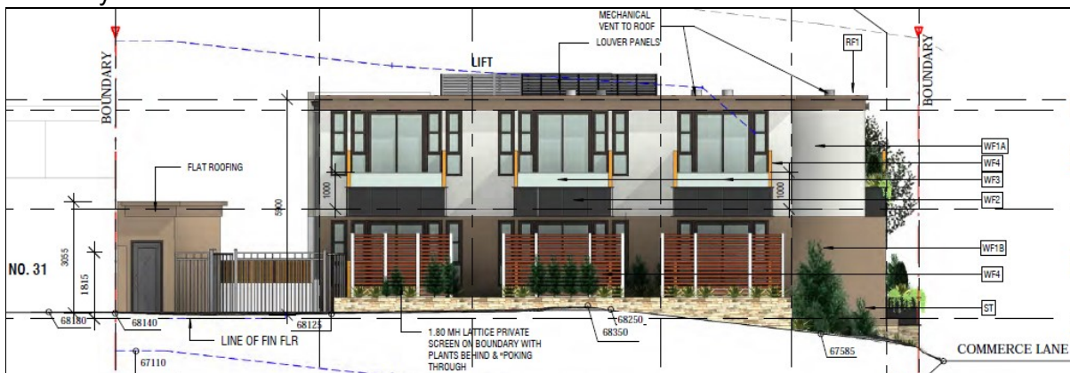
Image: Southern setback to Commerce Lane as per amended design to assist privacy and streetscape facing No.26 Nolan Place.
