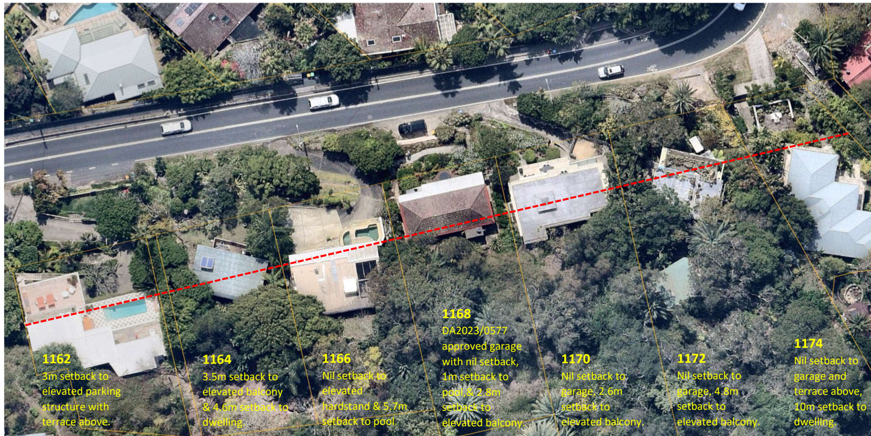
Figure 9 – Aerial image of Barrenjoey Rd with 10m front building line shown in the dashed red line Source: Nearmap and NBP
