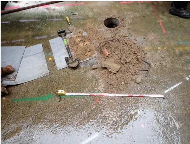
Figure 16 – Geotechnical investigation area, note mixed sandy fill removed from corehole (hand-augered), west of George Moncrieff Baron Wing.
