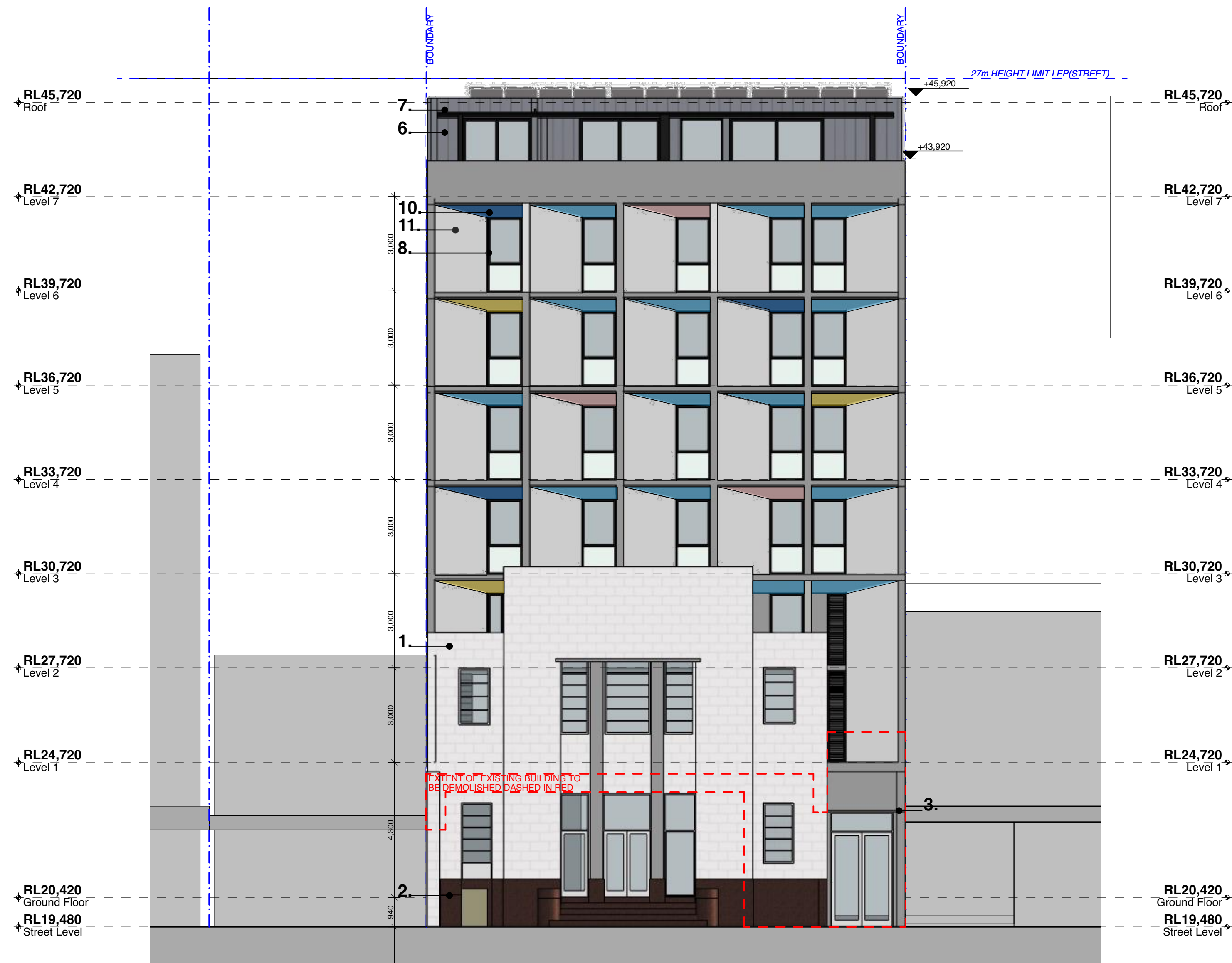
1 Southeast Elevation - Pittwater Rd Street Frontage 1:100
