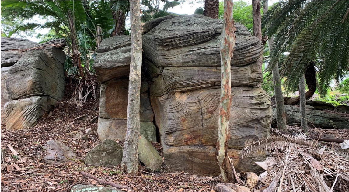
Photograph-7: Eastern view of boulder instability region, including the stacked boulder section to the left and large southern boulder to the right.
