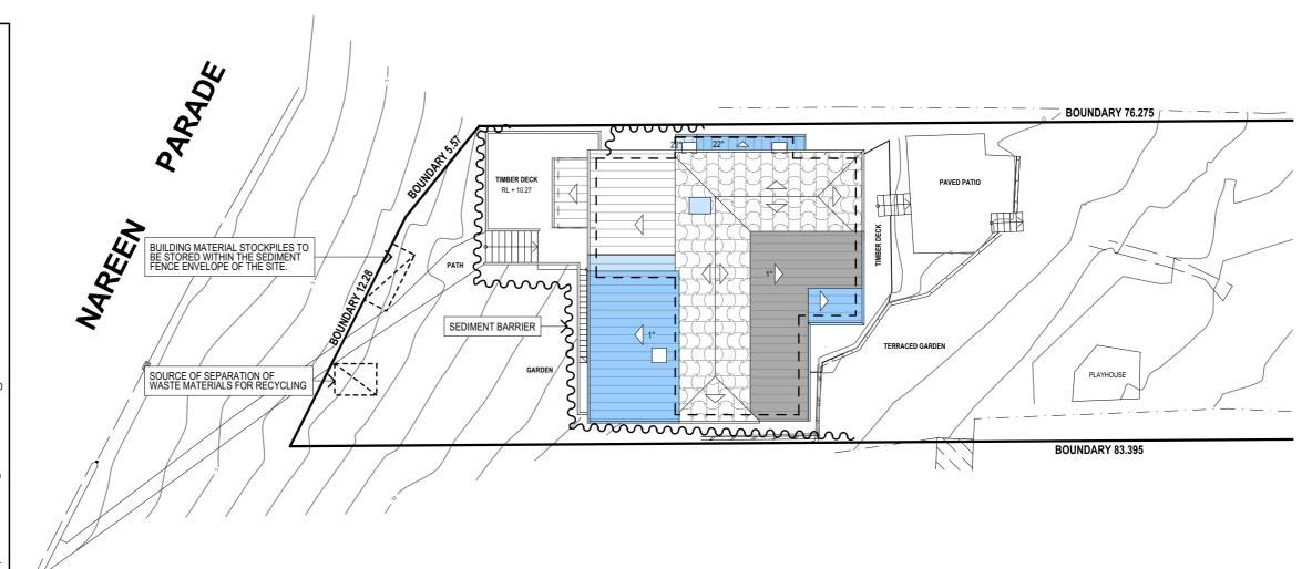
EROSION AND SEDIMENT CONTROL / WASTE MANAGEMENT PLAN
