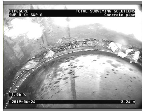
Photo: 1_4A, 00:01:39 2.24m, Breaking, some pieces are missing, at joint, length of break 100 , from 12 to 12 o'clock
