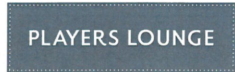
PL01 'Players Lounge' Wall Mounted Lightbox 1125x350mm Lightbox with push through LED dimensional letters and LED chaser light border, mounted to wall above rear entry.
