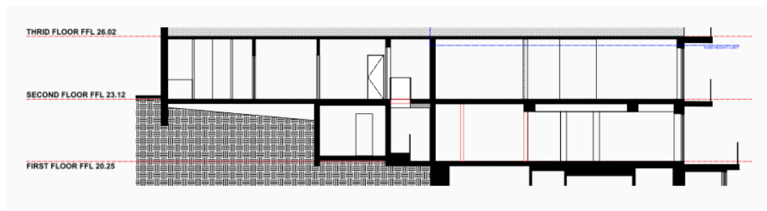
Figure 3: Extract from section showing height non-compliance
