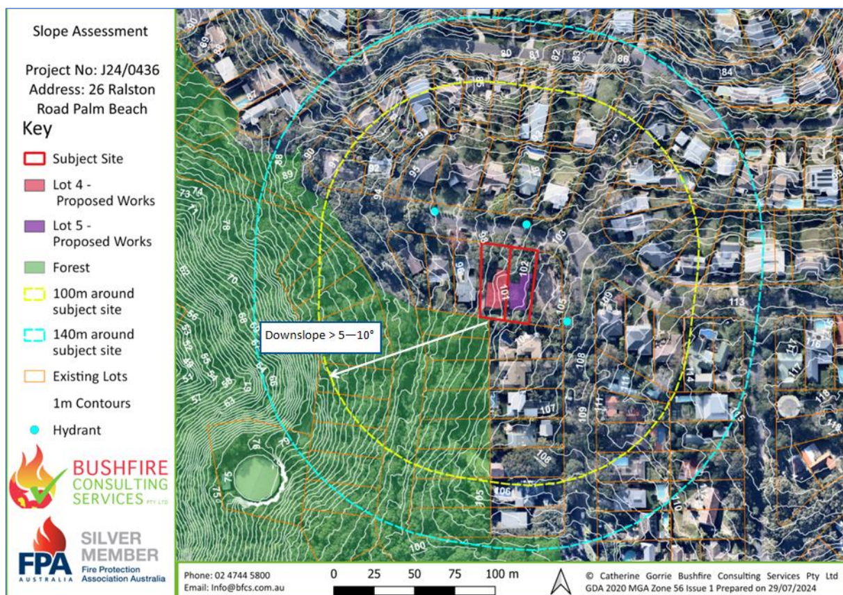
Figure 10. Slope Diagram. Source: NearMap (2024) and LiDAR (NSW Government 2024a) with overlays by BFCs P/L: Aerial Photography Date: 14/07/2024
