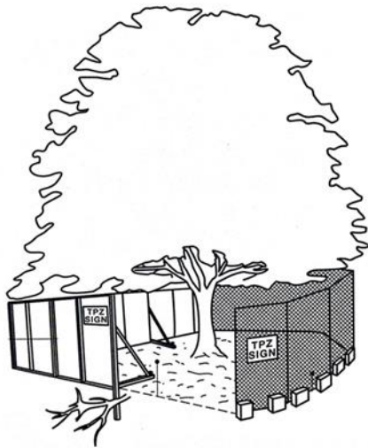
Tree protection fencing
