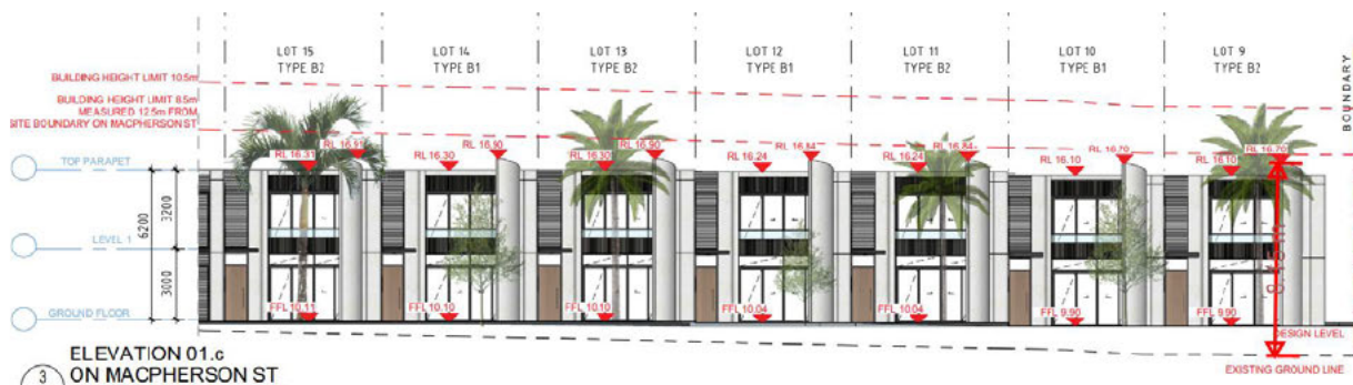
Figure 2: Excerpt of elevation 01.c from Architectural Plans for dwellings fronting Macpherson Street. A height line has been marked demonstrating that based on the existing ground levels, the maximum building height of Lot 9 Type B2 is approximately 8.15m.
