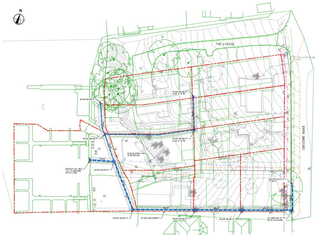
Figure 15: Stormwater Drainage Plan (BG&E)
