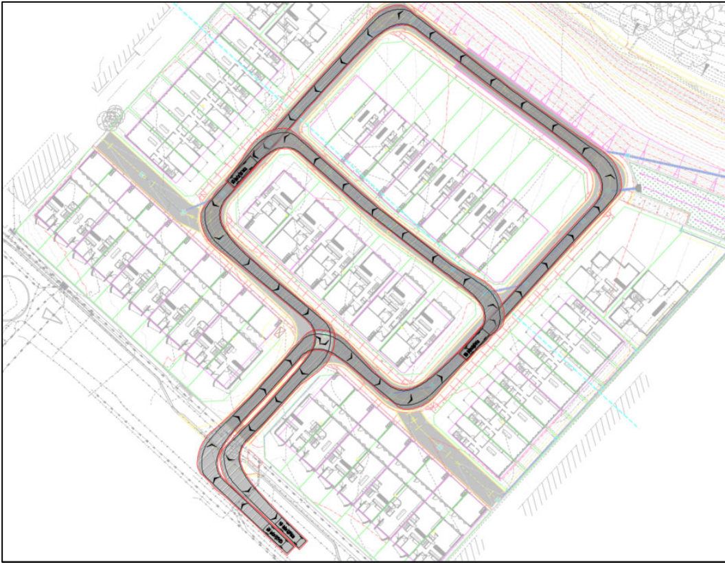
Figure 6 Swept path analysis – waste truck
